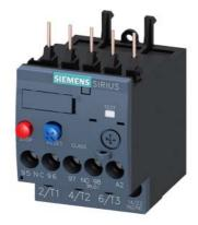
Overload relay 0.22...0.32 A Thermal For motor protection Size S00, Class 10 Contactor mounting Main circuit: Screw Auxiliary circuit: Screw Manual-Automatic-Reset
